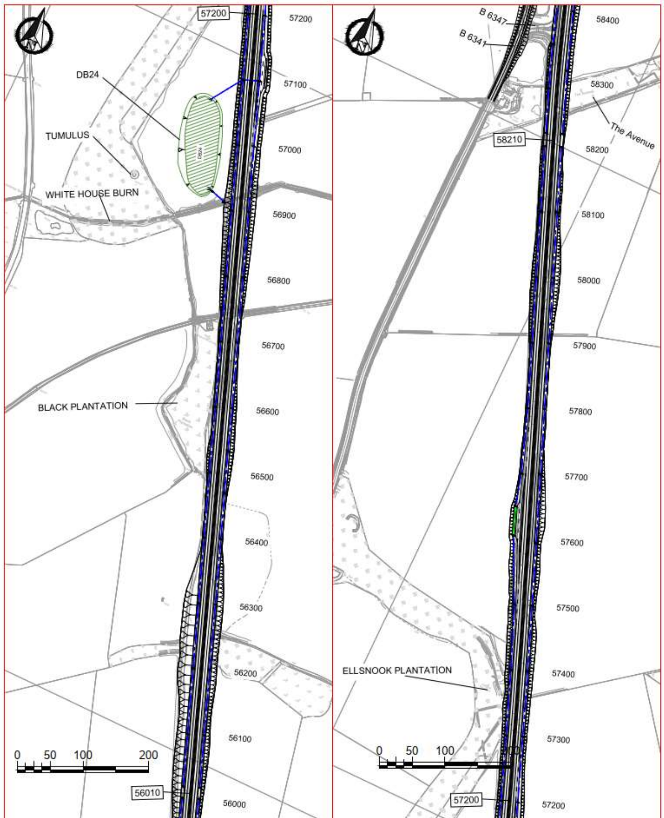
Figure 4-3 - Highway Drainage Layout and Detention Basin DB24
